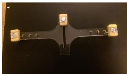
Figure 4 - Proses Track Laying Clamp
