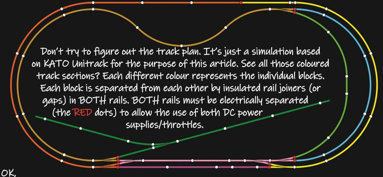
so how do we wire this thing? Go get a bunch of double pole - double throw center off toggle switches. You'll need one for each block. For Wagon Train we'll need 8. And a bunch of wire.
