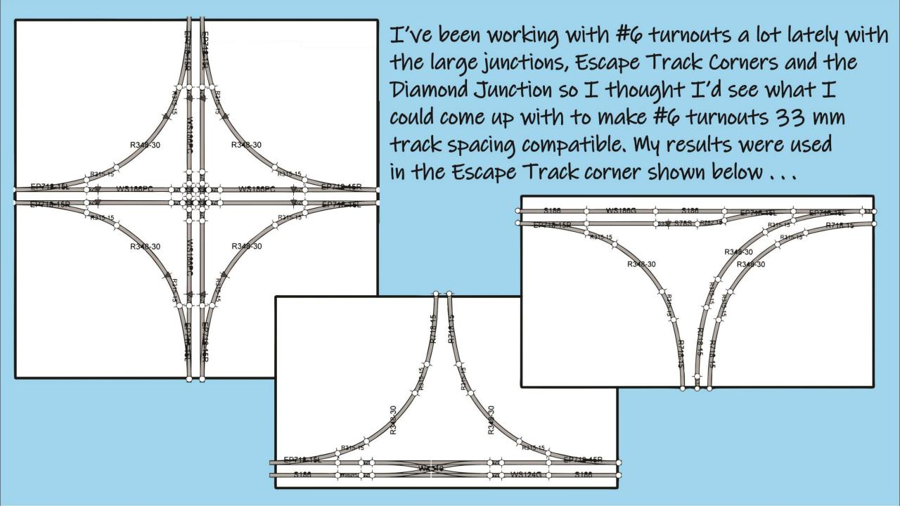
4.8.1. Use Kato Unitrack # 6 turnouts (part #20-202 & 20-203) whenever possible. Their use creates track spacing (49.5mm) that allows for easier placing of rolling stock on the track(s).
