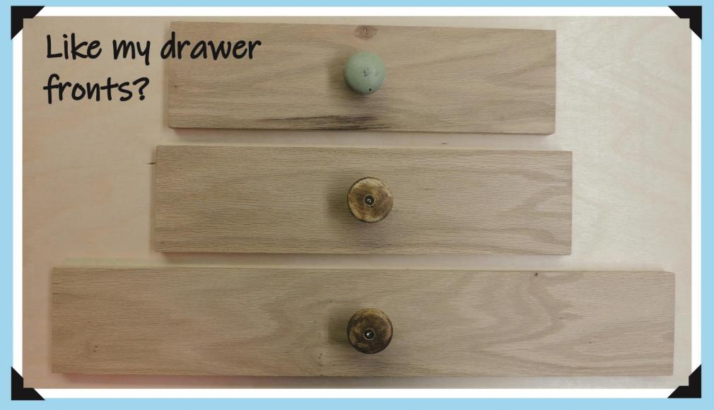
I purchased a short "project board" of 1x4 Oak (hardwood durability) and cut it into various lengths. The nominal 4 inch measurement is actually 3 1/2 inches. Just right! Added old knobs from a local ReStore making them very easy to handle setting modules.
