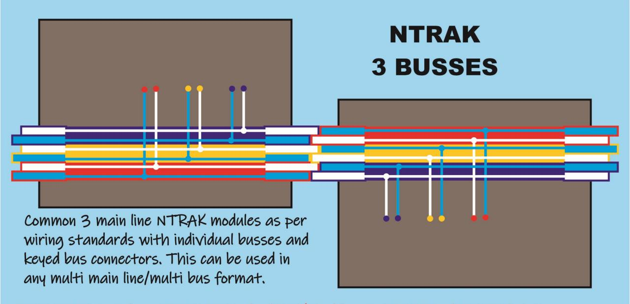
NOTE: NTRAK started as a FRONT, LEFT end and RIGHT end format with MALE and FEMALE Cinch Jones connectors. That, plus sky boards, limits module configuration. "Large T-TRAK" could be expanded to a 3 bus/track format.
