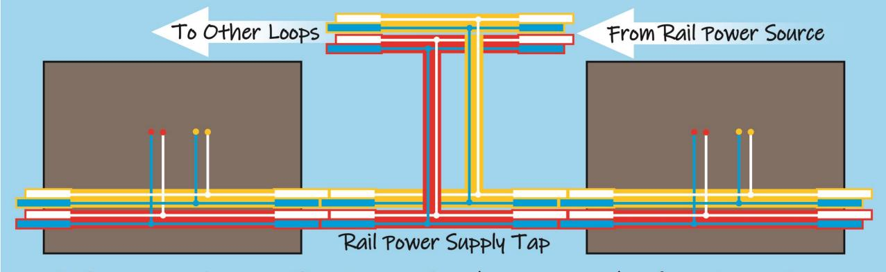
Rail power supply taps utilize the same keyed connectors and configuration as the module busses and can be inserted between any two modules. Long "extension cables" of any required length would be used from the rail power source to the rail power supply taps. Only 1 is required per loop/DC block/DCC district. Due to the independent nature of Yellow inside loops, taps will be necessary to chain supply the Yellow loops unless they have independent power sources (DC loop in a DCC layout).
