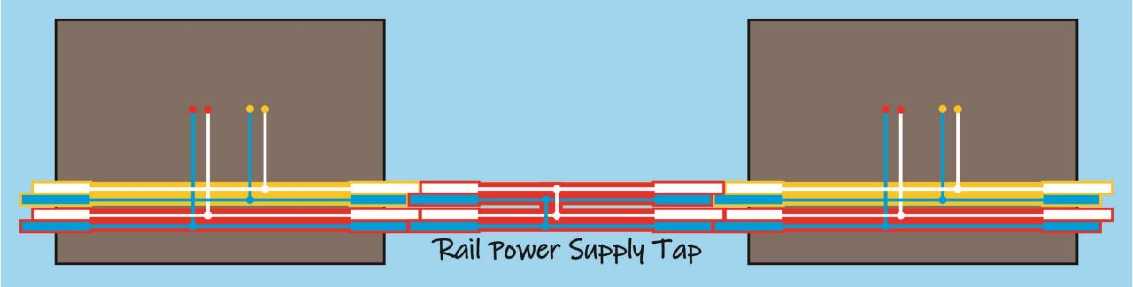
If a Yellow loop/track is to be powered by the same source as the Red track passing by a Rail Power Supply Tap connected to the Red Module Bus could be connected to the Yellow Module Bus to power the Yellow loop. (Single source DC or DCC)
