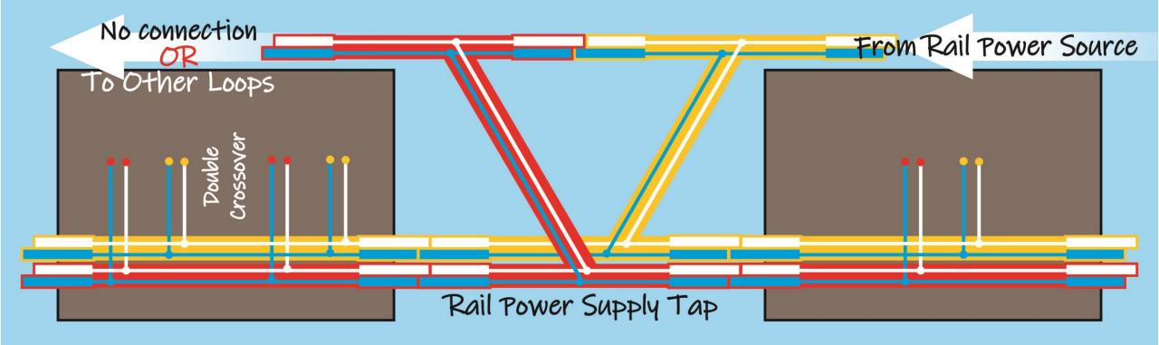
Since the Blue-White-Blue-White wiring standard is used the Red track and Yellow inside loop can be fed from the same Rail Power Source by connecting the Red and Yellow Rail Power Supply Taps together, unless the Yellow loop requires a separate power source (DC loop in a DCC layout).
