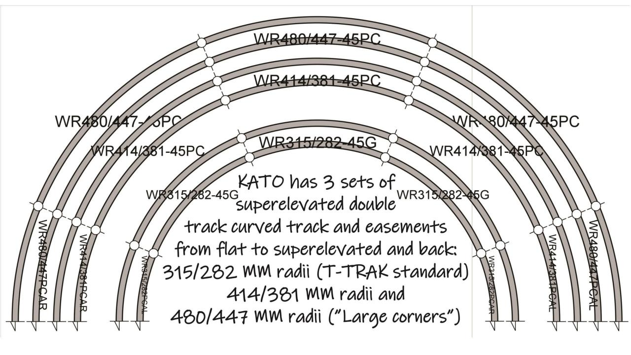
Although an "end cap" 180 degree corner of 480/447 MM superelevated curved track is possible it would be substantially larger than the 315/282 MM one shown here.
