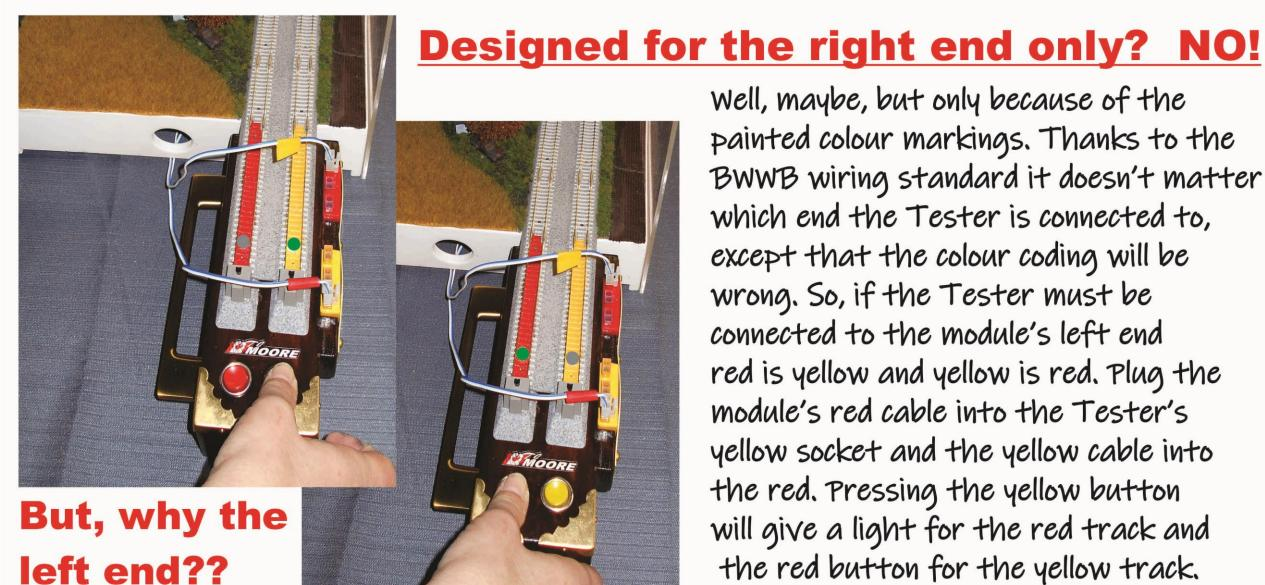
Well, maybe, but only because of the painted colour markings. Thanks to the BWWB wiring standard it doesn't matter which end the Tester is connected to, except that the colour coding will be wrong. So, if the Tester must be connected to the module's left end red is yellow and yellow is red. Plug the module's red cable into the Tester's yellow socket and the yellow cable into the red. Pressing the yellow button will give a light for the red track and the red button for the yellow track.
