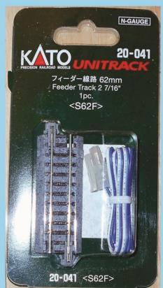
The feeder wire connecting plugs for the 62mm single track Feeder Tracks can only be connected to the track piece one way. Using single track pieces the BWWB wiring standard can be created by reversing the position of the two tracks relative to each other with the blue wire supplied rails on the outsides.
