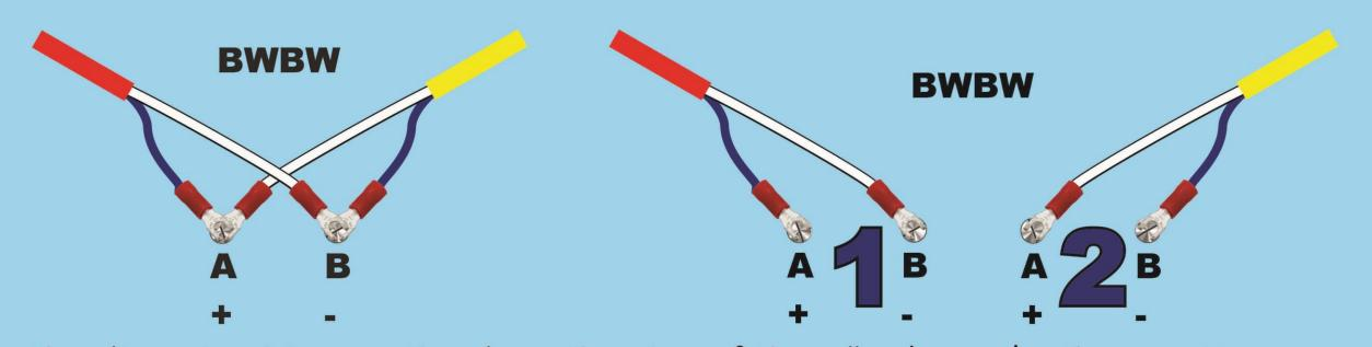
The alternate wiring practice places the wires of the yellow bus under the opposite power supply terminals of the red bus creating a pseudo BWBW wiring condition at the rails allowing the use of crossovers. IF multiple power supplies are used connections must be identical on all power supplies. Separate power supplies may be used for each bus.
