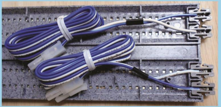
A pair of Terminal Unijoiners allow installation anywhere two pieces of track come together and allow for placement in the required BWWB positioning. They can be used in corners or next to turnouts where the 62mm straight track pieces can't be installed. Due to the wiring they can not be used at the track ends of a module. Bury them inside the module's trackage between any two pieces of track such as between the 62 and 248mm track pieces of this single module.
