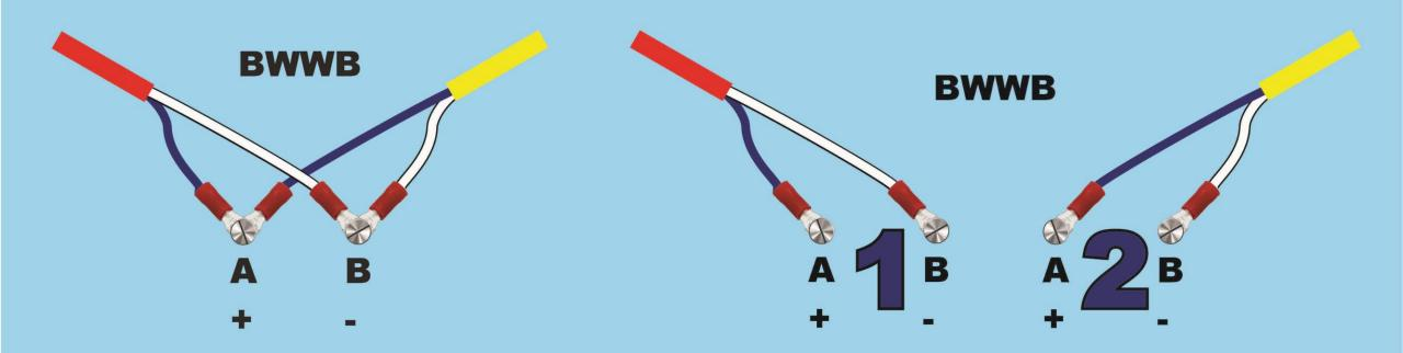
Standard T-TRAK wiring practice places the blue wires of both the red and yellow busses under the same power supply terminal and the white wires of both busses under the other power supply terminal. IF multiple power supplies are used connections must be identical on all power supplies. Separate power supplies may be used for each bus.
